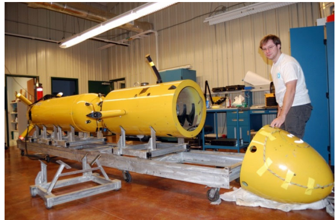
Figure 1. The Eagle Ray Autonomous Underwater Vehicle has a large payload capacity making it a suitable test bed for the development of new sensors and instruments.
