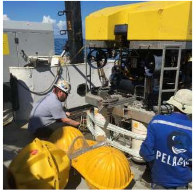
Figure 7: Equipment array cradle being mounted to the ROV
