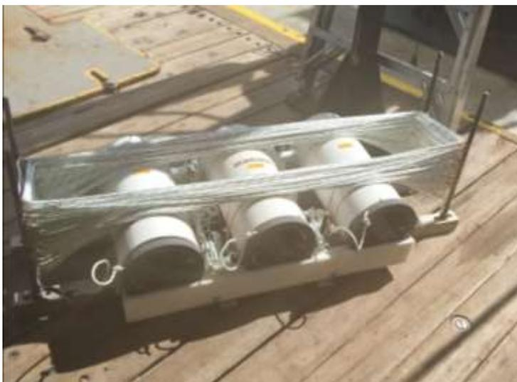
Figure 5: Microbial experiment array on cradle and prepped for deployment
