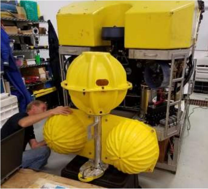
Figure 6: Lander prototype being test mounted on the ROV
