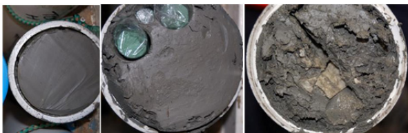
Figure 5. (left) Undisturbed section of core 3. (middle) Section of JPC-006 showing sampled section. Note blisters of gas appearing on exposed surface. (right) Hydrate comprises a significant fraction of this section of JPC-001, opened nearly 2 hours after retrieval. Note large chunks of hydrate.
