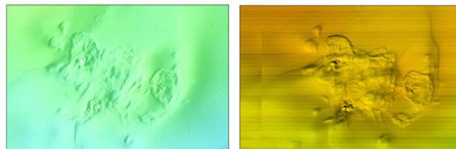
Figure 1. Comparison of the seafloor bathymetry map of MC118 from a commercial standard AUV survey (left) and the same image following the application of MMRI in-house post-processing (right).
