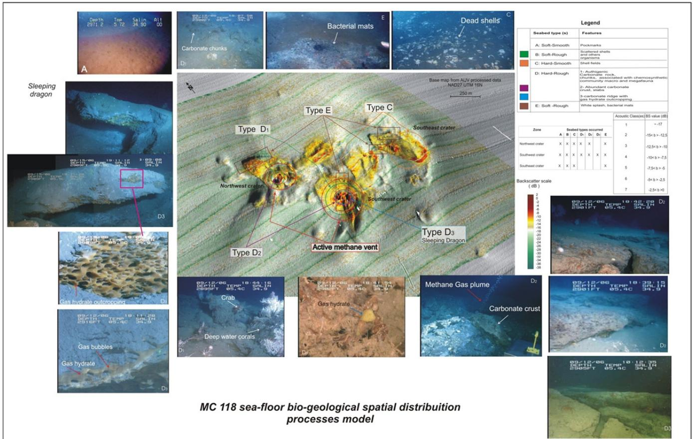
Figure 3. Composite illustration of the bio-geological processes active at Woolsey Mound (MC118). The model has been created integrating multibeam data, seafloor reflectivity, grab samples, video and camera surveys.
