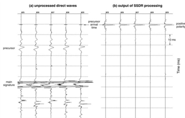
Figure 2. Water gun signature processing. The raw water gun far field signature (a) is a broad and inconsistent seismic pulse; phase conjugation processing (b) collapses the pulse into a narrow signal increasing the vertical resolution, Macelloni, et al., 2011.
