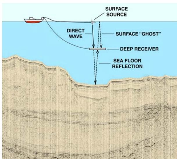
Figure 1. Illustration of SSDR recording geometry
