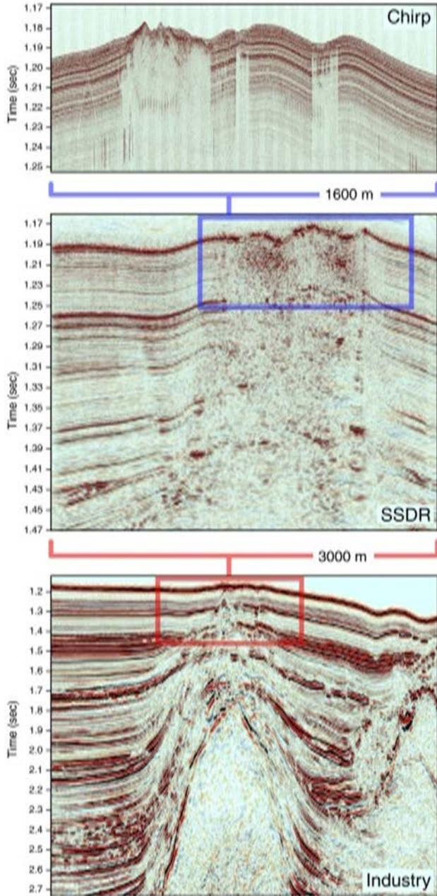
Figure 3. A multiple seismic data resolution approach provides maximum resolution to depth. High-resolution chirp profile (top) details the top .04 sec (~30mbsf), the SSDR (middle) shows the best resolution of the next .40 (~300) and the low resolution industry
