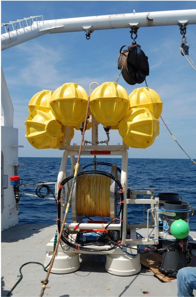
Figure 2: The ROVARD on the back deck of the R/V Pelican. Note recovery lift line spooled up in the center of the platform and the series of yellow glass floats that ascend through the water column once the acoustic releases are triggered.
