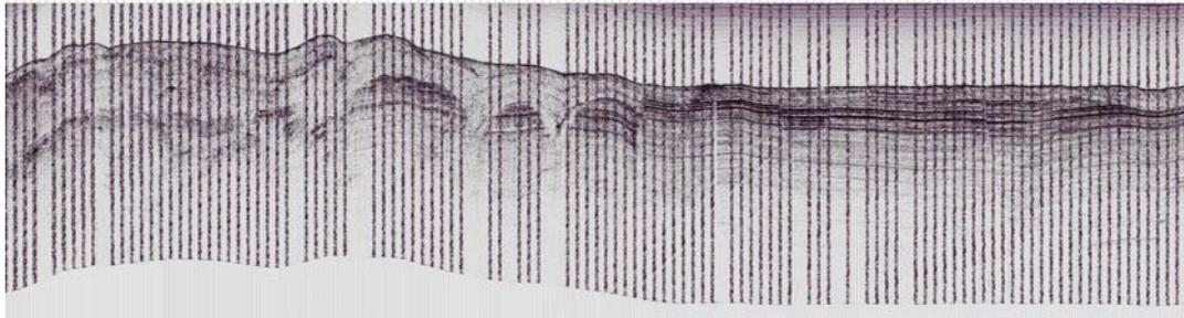
Figure 3. Sub-bottom profile through gas expulsion feature in Ewing Banks 873, Gulf of Mexico, acquired with the Polarity Preserving Chirp Sub-bottom Profiler.
