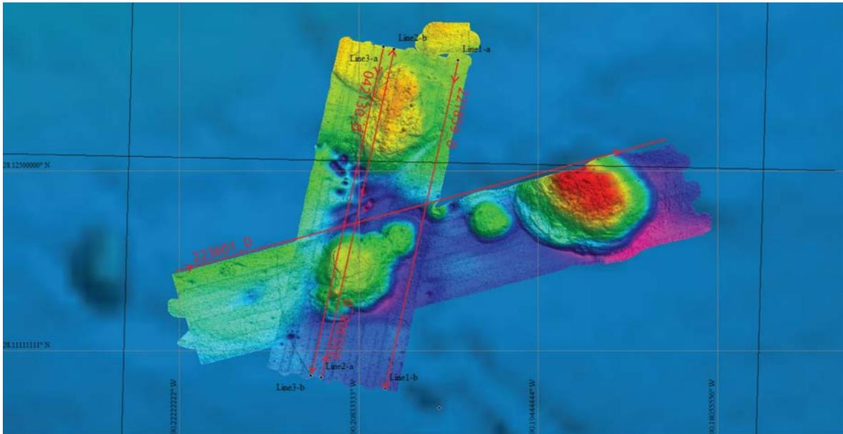
Figure 2. High-resolution bathymetric image of Ewing Banks 873, Gulf of Mexico, acquired by the Eagle Ray AUV. Note the mud volcanoes (red to orange areas) and the pock marks (dark blue to magenta circular areas) gas expulsion features on the sea floor.
