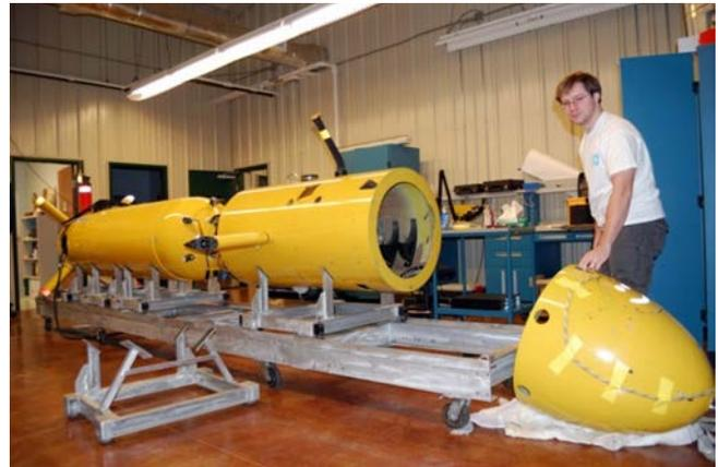
Figure 1. The Eagle Ray Autonomous Underwater Vehicle has a large payload capacity making it a suitable test bed for the development of new sensors and instruments.
